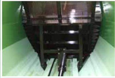
**The bulkhead** is operated by a multi-stage telescopic ram. The HAWE CSW experiences very little wear because moving parts are reduced to a minimum
