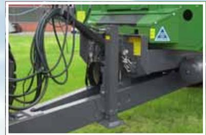
**Hydraulic parking stand** and hydraulic drawbar suspension.
