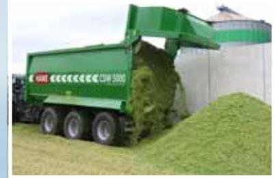
All HAWE CSW have a high level of stability due to the low center of gravity, even when unloading on side slopes and in low buildings where headroom is limited.
