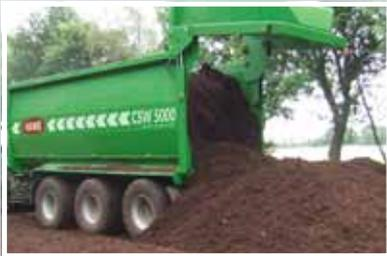
HAWE CSW push-off trailers are suitable for the transportation of various goods. Heavy or damp loads can also be safely and quickly unloaded.
