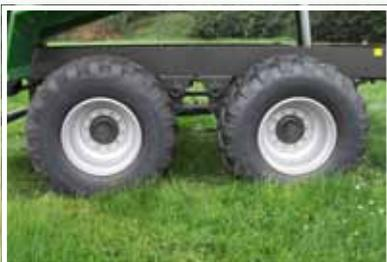
The standard equipment includes heavy running gear with **parabolic suspension**, BPW axles and generously sized brakes.
