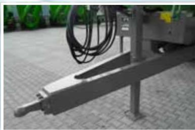
Hydraulic parking stand and mechanical **drawbar suspension**.
