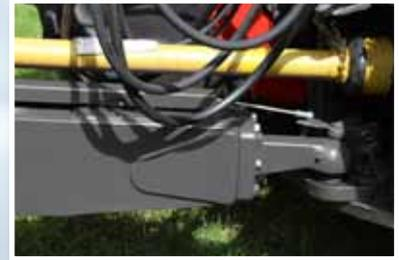
The **positive steering system** is controlled by a Bowden cable.
