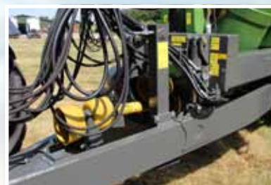
Hydraulic parking stand and hydraulic drawbar suspension.
