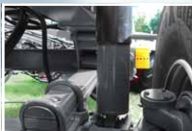
Running gear with hydraulic suspension available for all Tandem and Tridem chassis.
