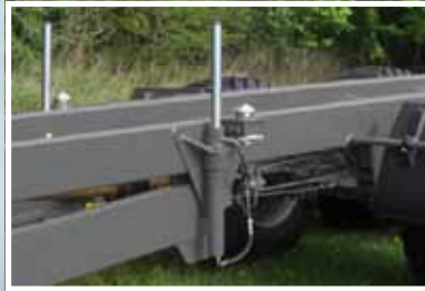
Lifting rams to remove and install the different bodies.
