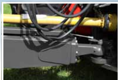
The positive steering system is controlled by a Bowden cable or electronically controlled.
